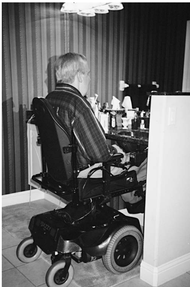
Figure 26-20 This gentleman uses a powered vertical up/down seat on a power-based wheelchair to allow better height and close approach to the sink for grooming activities.
