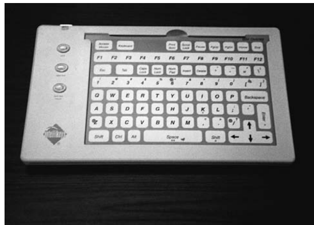
Figure 18-8 Intellikeys keyboard allows easy modification when the user needs large keys or decreased sensitivity.
