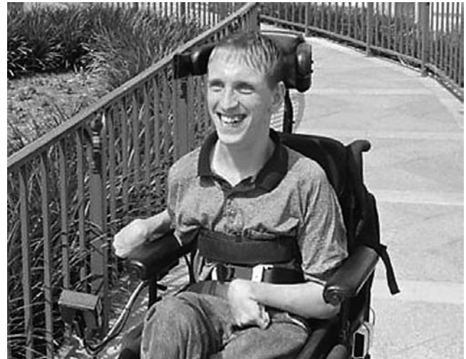
Figure 17-7 College student uses a power wheelchair controlled with proximity switches in a head array. The display in front of right armrest provides feedback regarding drive selection, electronic aids to daily living (EADL) functions, and battery level. A switch on the right side of the head array permits selection of drive and EADL functions. (Courtesy of Adaptive Switch Laboratories, Inc., Spicewood, TX.)
