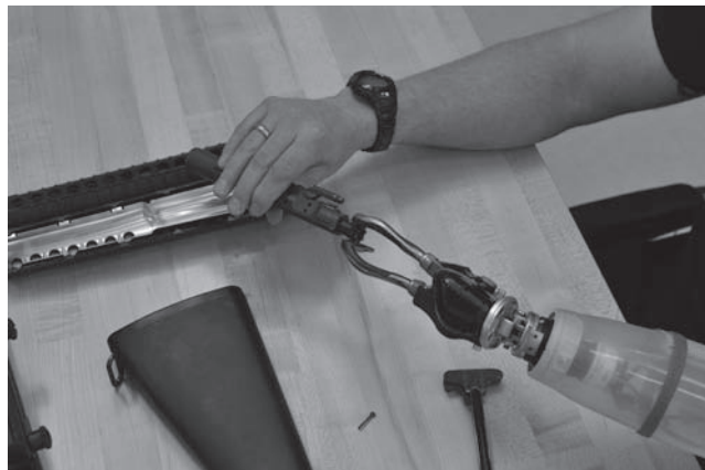
Figure 41-25 Assembling a mock weapon using a myoelectric prosthesis with a wrist rotator and wrist flexion component. This is a meaningful and purposeful activity for service members.
