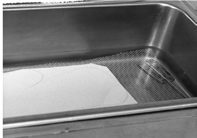
Figure 16-13 Heating the thermoplastic.
