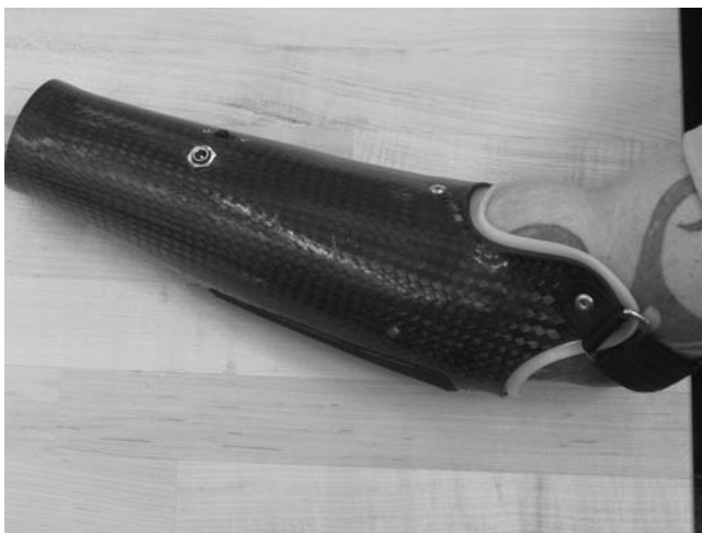
Figure 41-5 Myoelectric transradial prosthesis shown with a carbon fiber socket and without a terminal device.
