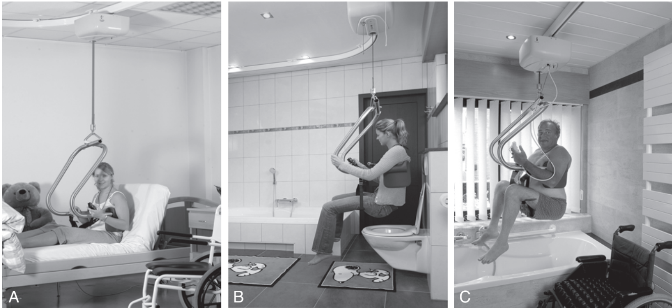
Figure 26-6 Motorized lifting systems assist physically challenged individuals or their caregivers in transfer goals for accessing the bed, shower, tub, toilet, or pool. (Courtesy of SureHands Lift & Care Systems, Pine Island, NY.)
