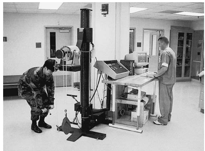
Figure 28-9 BTE Work Simulator used for dynamic strength testing.
