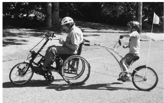
Figure 17-8 A father uses a cycling apparatus attached to his everyday-use manual wheelchair for outdoor activity with his children.
