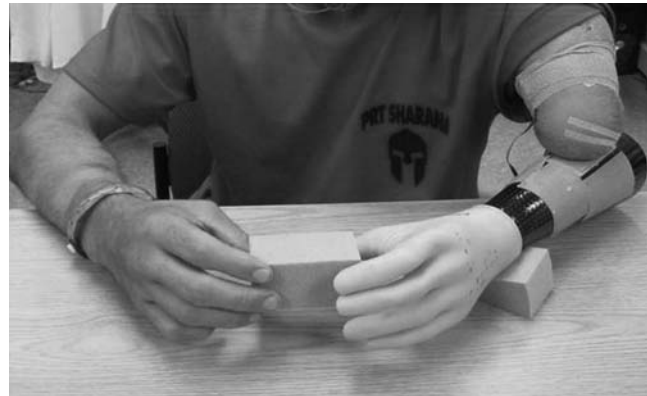
Figure 41-9 Myoelectric site training during the preprosthetic training phase at midline. The electrodes are placed on the patient’s biceps and triceps myosites. The electrode leads are connected to a universal carbon fiber demonstration socket with an Ottobock System Electric Hand (Minneapolis, MN) with a standard hand shell covering the terminal device. Use of the demonstration socket allows the patient to experience what it is like to control an actual myoelectric terminal device. This patient is practicing grasp and release with a foam block; use of this type of object is often for practicing proportional control during grasping.
